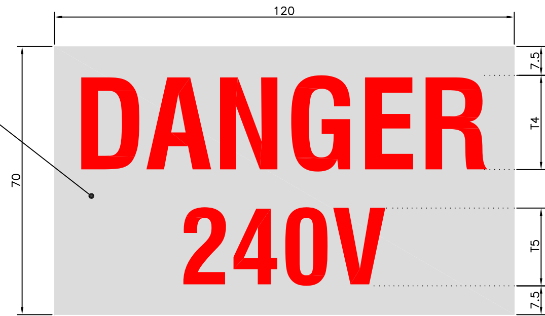
WARNING LABEL 2 'DANGER 240V'
